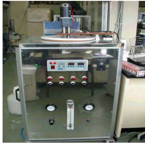
Fig. 2. Large lab-scale modified electrochemical decontamination system
