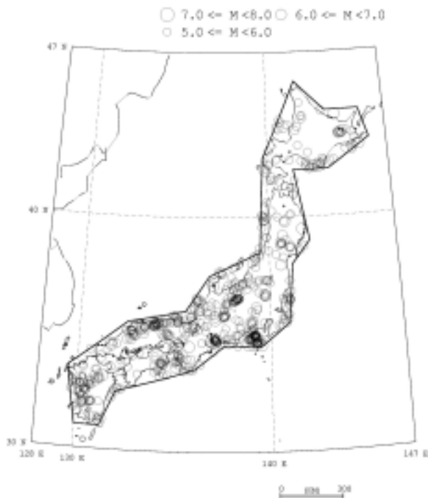
Figure 2 Source area model and distribution of epicenters of inland earthquakes
