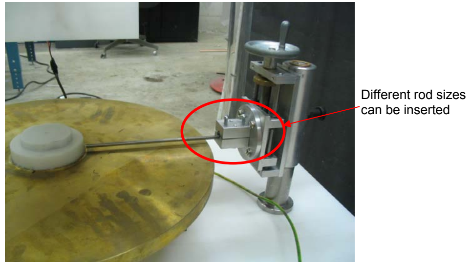
Figure 36: Modified design of the lay-down tube, which can carry all rod sizes up to \text{Ø}10\text{mm}
