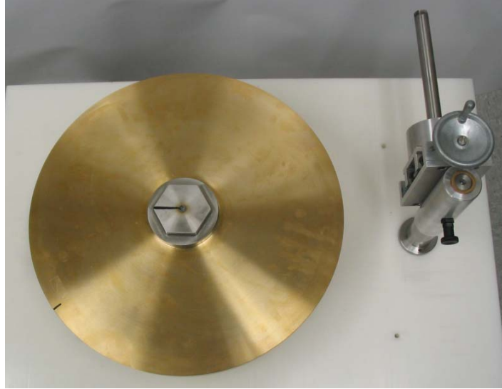
Figure 26: Tube can be swung for better access to the disc and fiberweb after web formation is completed (e.g. remove web)
