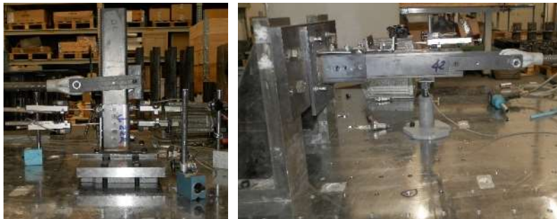
Figure 7. Tests of the foot connectors in in Pz, Py and Px direction.
