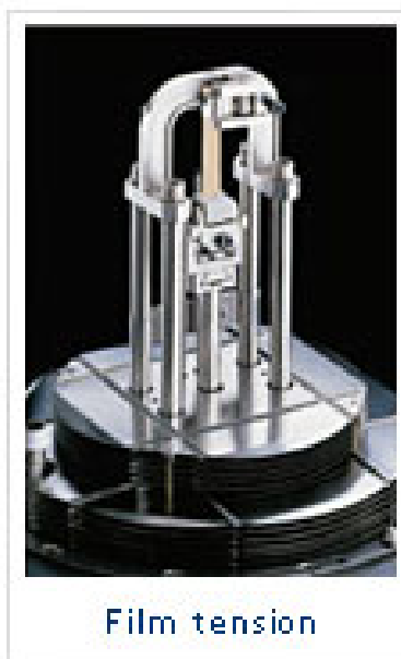
Figure 3: Custom submersion clamps for DMA experiments
