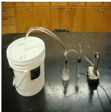
Figure 3-11 Schematic of air sampling system used in the chamber study
