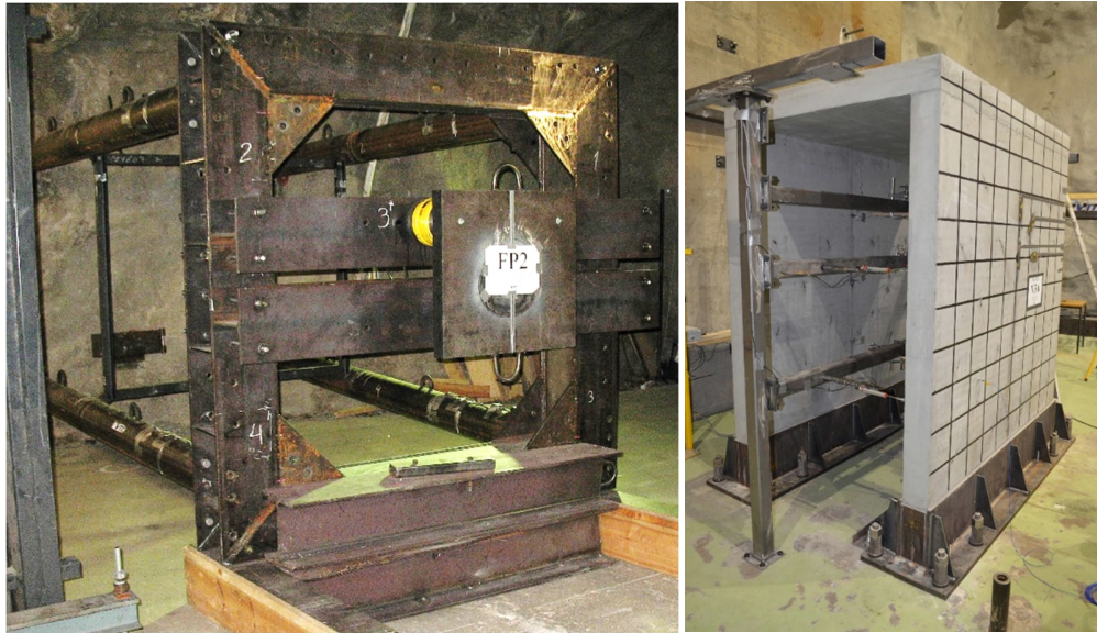
Figure 4. Left: Force plate test set-up. Right: Vibration test mock-up V3 (right) ready to be tested.
