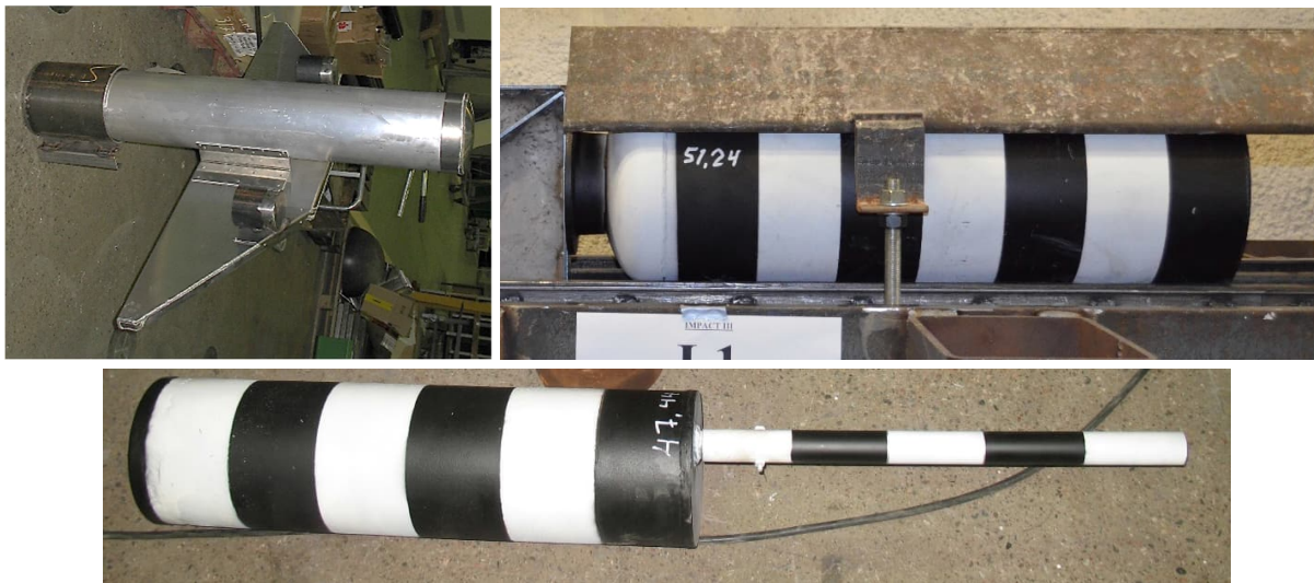
Figure 5. Top left: An aircraft model projectile used early in the test program. Top right: A water filled projectile maximizing the water mass. Bottom: A hard projectile.
