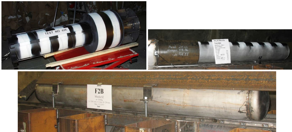
Figure 6. Top left: A soft projectile-piston system made out of threaded pipe. Top right: An aluminium projectile with heavy steely back part. Bottom: A stainless steel projectile.
