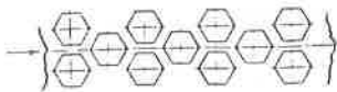
Fig. 4: Single rows of core elements as assumed in the PEC core calculations with the computer program CORALIE
