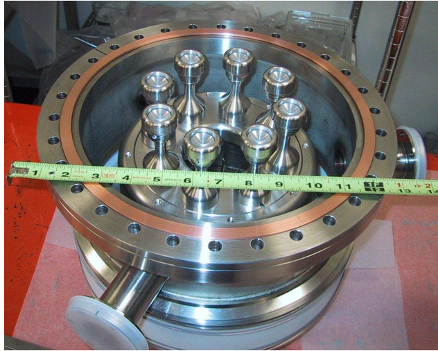
Figure 3.2.1: Electron gun under construction
