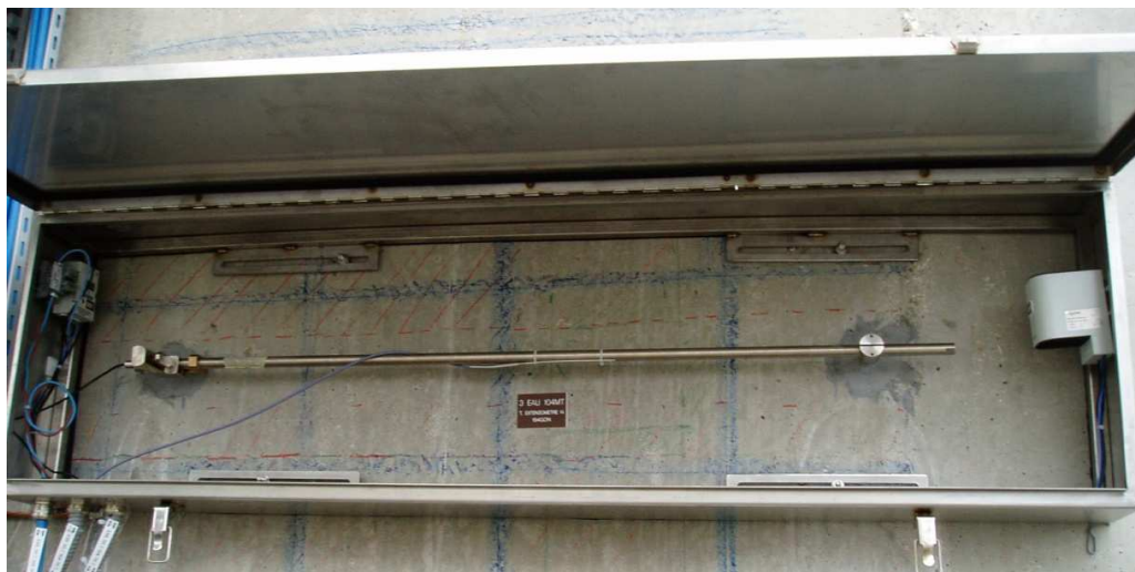
Fig.5: Surface strain meter installed on site. The displacement sensor is installed on the left hand end of the 1 m Invar bar.
