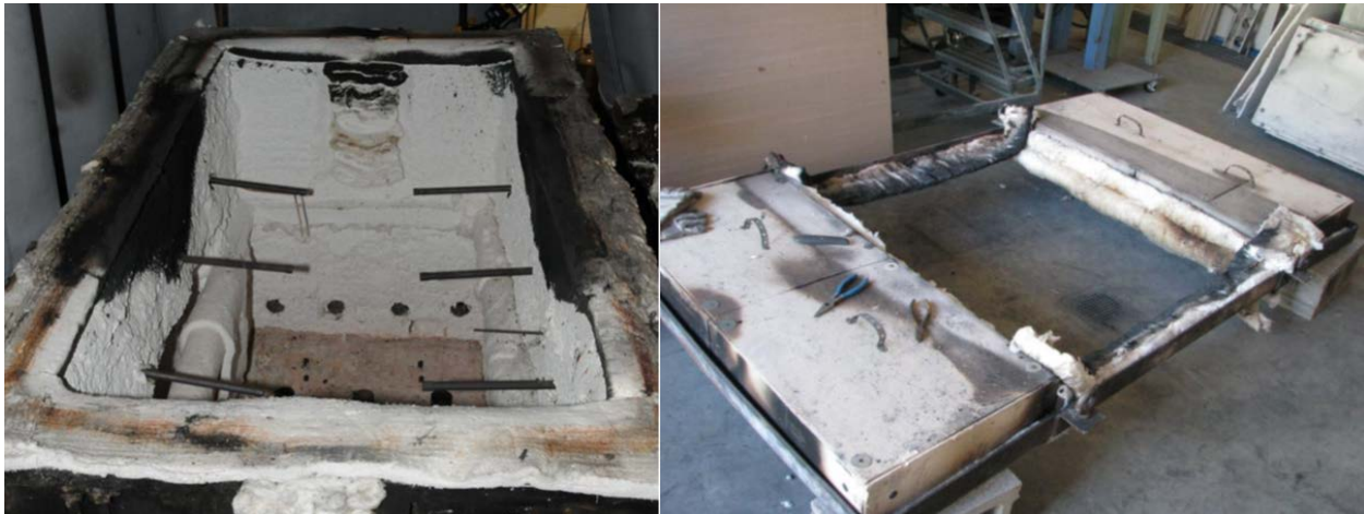
Figure 4.9. Intermediate-scale horizontal furnace (Left) and specimen frame (Right) (Courtesy of Forest Product Laboratory).
