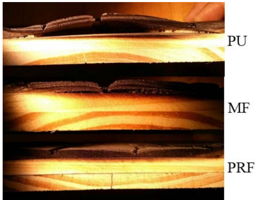
Figure 4.13. Previous unpublished fire test results: PU glued sample (top) had severe delamination; MF (middle) had less delamination; PRF had no delamination.
