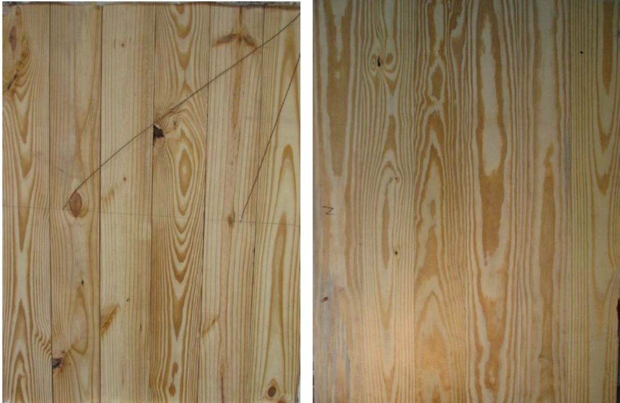
Figure 4.23. Comparison of exposed surfaces prior fire test of sample 3 from Group A (left, non-edge-glued) and sample (5) from Group B (edge-glued). (Courtesy of Forest Product Laboratory).
