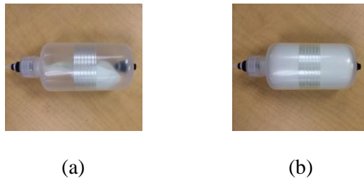
Figure 16. Elastic bladder inside ballast tank in (a) deflated and (b) inflated states.
