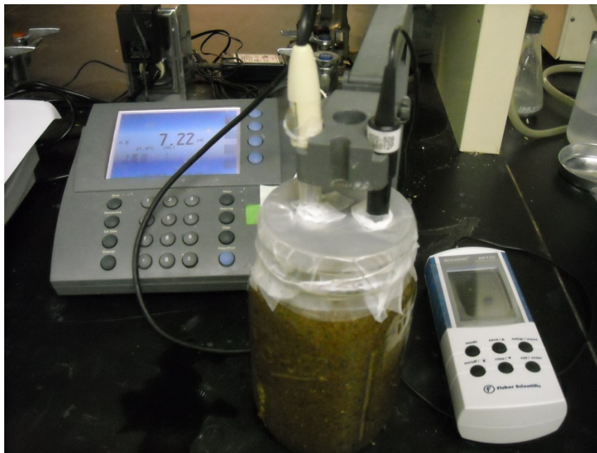
Figure 3-1 Experiment design of dissociation constant. At left is the pH electrode, and at right is ammonia electrode)
