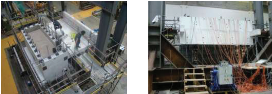
Figure 4: Static cyclic test set-up (Model-1)
