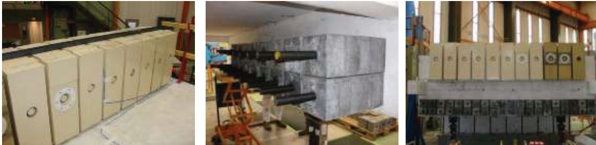
Figure 3: Additional masses fixed on Model-2
