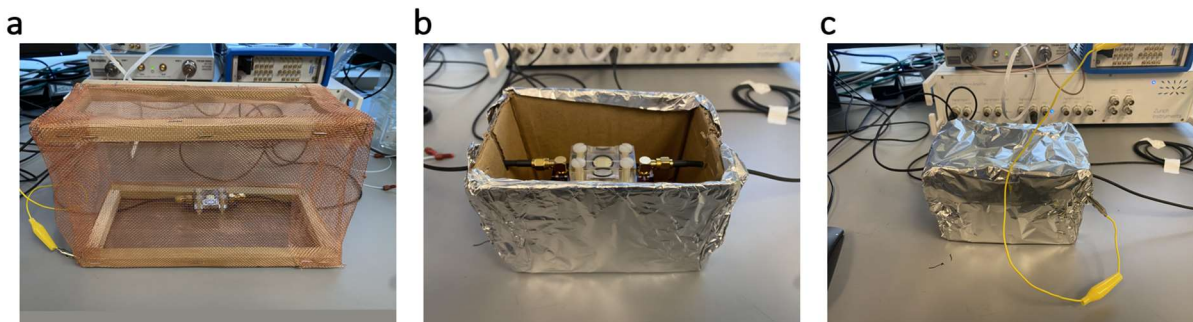
Figure 19. Faraday cage setups used for the QCM biosensor. (a) Copper mesh screen surrounded by a wooden frame. (b) Open cardboard box encased in thick aluminum foil. (c) Closed cardboard box surrounded by aluminum foil.
