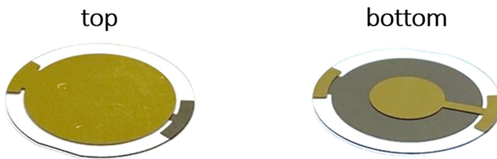
Figure 8. AT-cut QCM purchased from openQCM. Top and bottom of the crystal used for QCM binding experiments [45, 46]. The larger top electrode contacts the liquid sample, and the electrodes overlap in the middle which creates a sensitive region.
