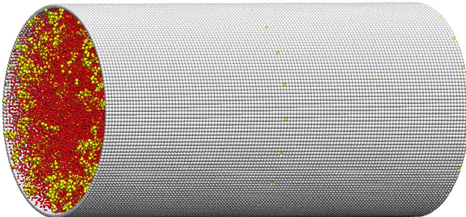
Figure 3.2 Snapshot from a MD simulation of the polymer grafted cylindrical nanopore. Color-coding: red (fluid atoms), gray (wall atoms) and yellow (polymer).
