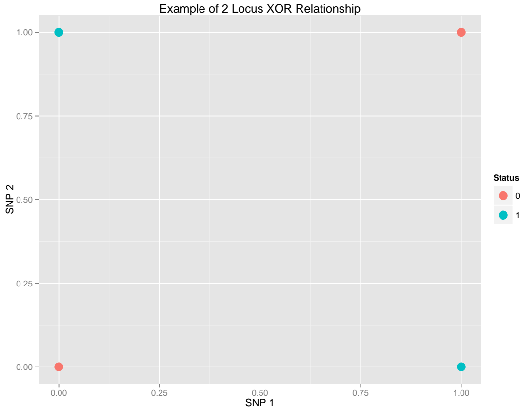
Figure 1.1: Example of a 2 locus epistatic interaction. Trait status is determined by an XOR operation of SNP 1 and SNP 2. Note there does not exist a way to separate the two classes with a linear decision rule.
