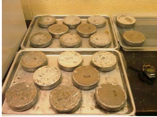
Figure 3.4 - Test Setup for Measurement of the Rates of Absorption of Water
