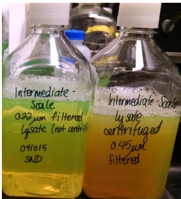
Figure 5.6. Photograph illustrating the visual difference in the same intermediate-scale lysate prepared using the current clarification process (right) and the direct 0.22 \mu\text{m} filtration process mimicking large scale (left) prepared on the same day.
