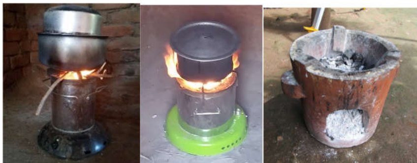
Figure A2. Improved stove technologies tested in the Malawi field campaign. L to R: Philips, ACE-1 and Chitetezo Mbaula . Pictures by A. Grieshop and P. Jagger ( Chitetezo Mbaula ).
