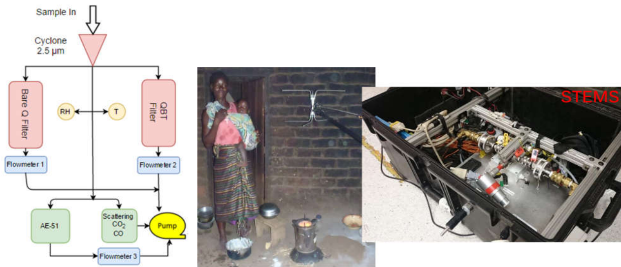
Figure A4. STEMS-1G Schematic and setup in the field. Each of the flowmeters have valves downstream for flow control (not shown).
