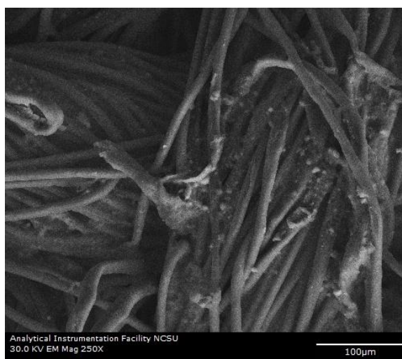
Figure 4.29: SEM Image of 25.0%THPC + 15.0% Urea + 0.5% TEOS + 9.0% TiO 2 Laundered Poly/Cotton Fabric
