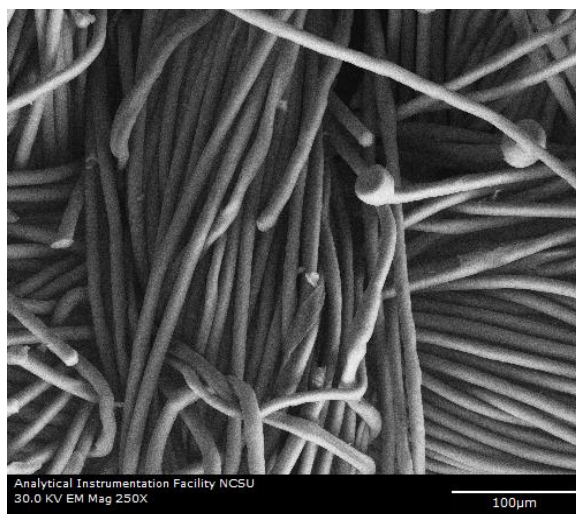
Figure 4.18: SEM Image of 25.0%THPC + 15.0% Urea + 0.5% TEOS + 3.0% TiO 2 Cotton Fabric
