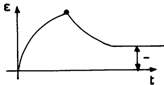
Permanent strain observed in real materials.
