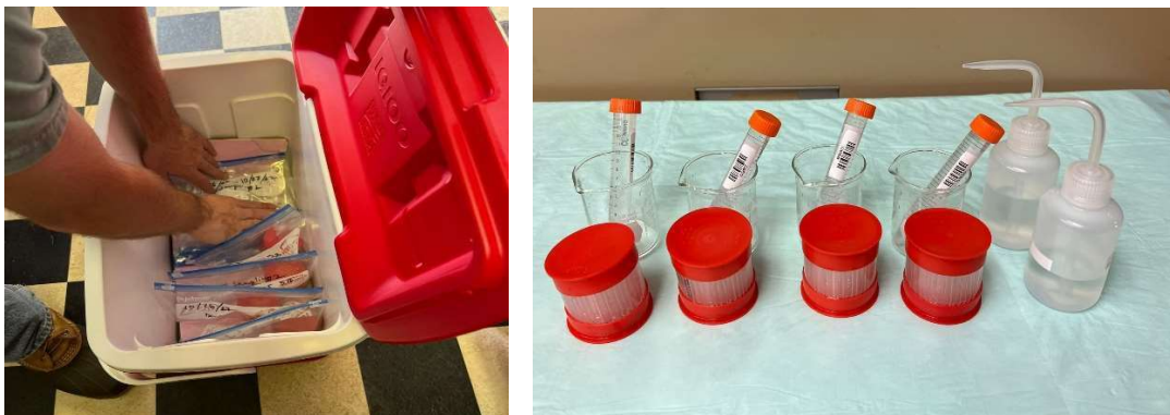
Figure 2.11. Storage of filters and denuders for transportation (left) and denuder samples after extraction in vials (right)
