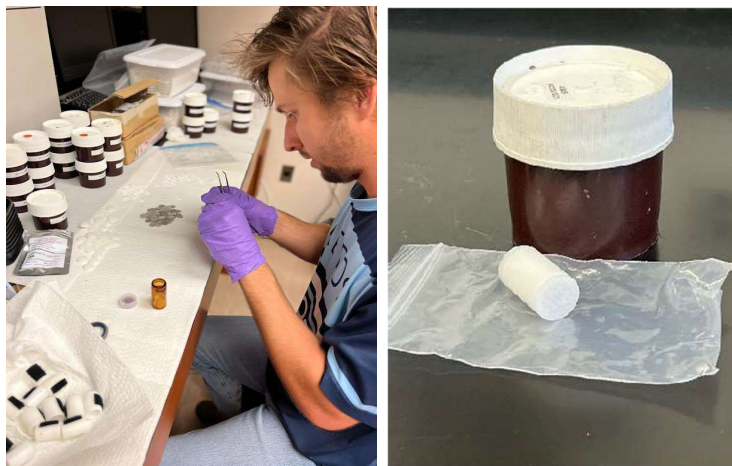
Figure 2.8. Assembling passive samplers (left) and Ogawa airtight storage container (right)
