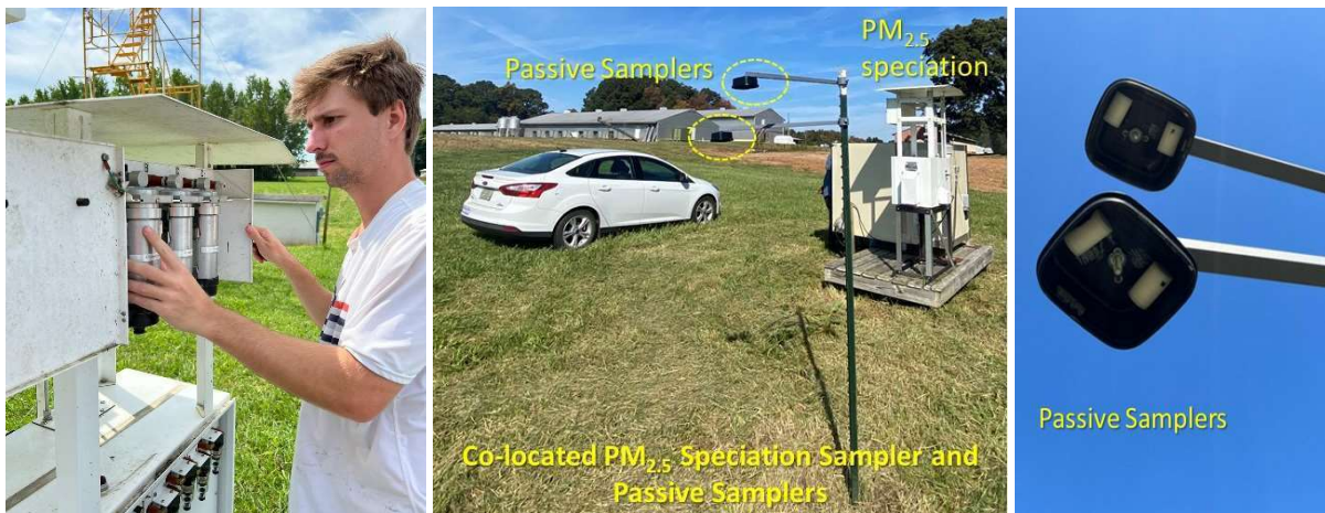
Figure 2.10. Illustration of PM 2.5 speciation samplers (left), co-located samplers (middle), Ogawa passive samplers with replicates (right)
