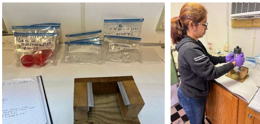
Figure 2.9. Installing filters to the cartridges in the field mobile lab
