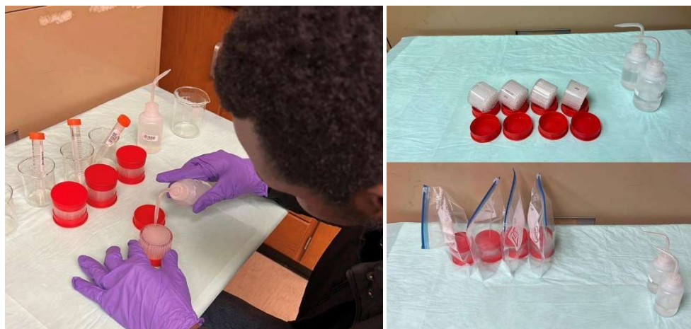
Figure 2.6. Application of 2% citric acid solution to coat honeycomb denuders
