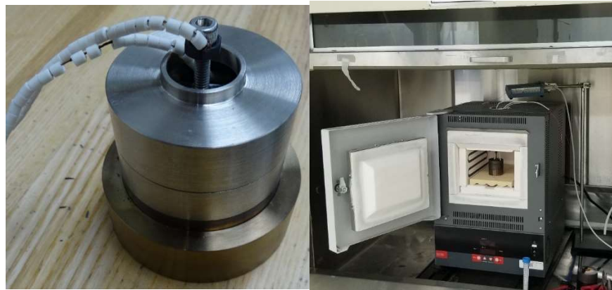
Figure 1. Full sensor housing assembled with attached signal wires, on benchtop (left) and connected in furnace (right)
