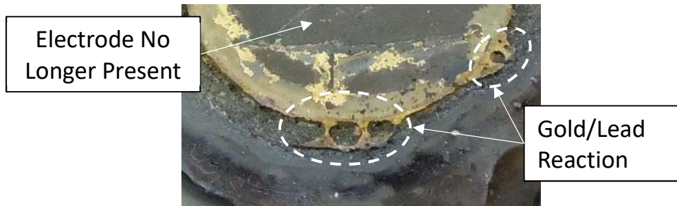
Figure 4. Lead reaction with gold electrodes on the piezo
