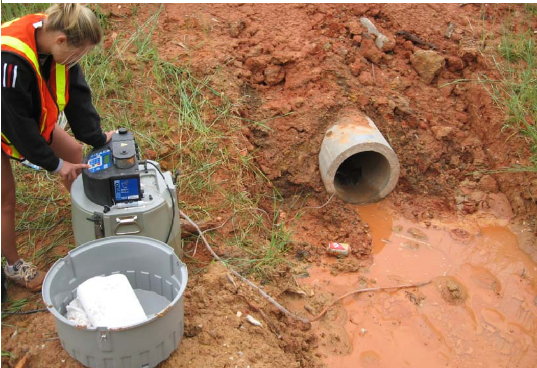
Figure 12. Effluent from Standard 10-year Trap with standing pool is released from this pipe. The Manning equation was used to install and program the sampler.
