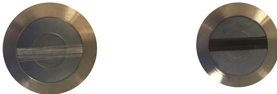
Figure 3.3 WAXD samples of pure polymer fibers (left) and PVOH-10% MNPs magnetic fibers (right).
