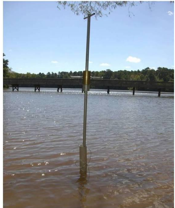
Figure 4.1 Left: Cook's Millpond sediments being sampled at a bank outcrop; Right: Geo-corer set up for coring at Yates' Millpond.
