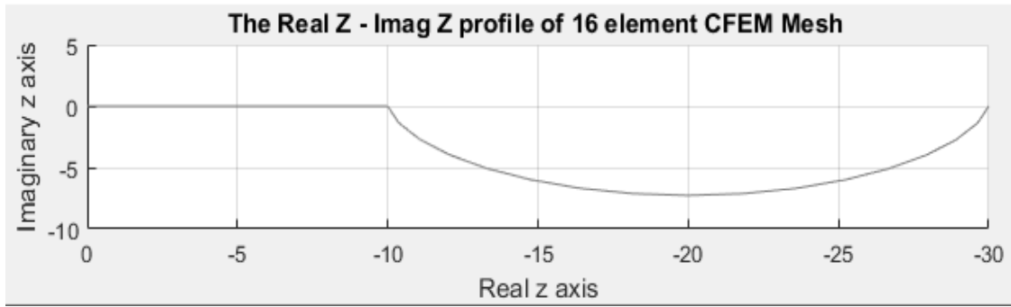
Figure 2-9 Bending of mesh into complex plane
