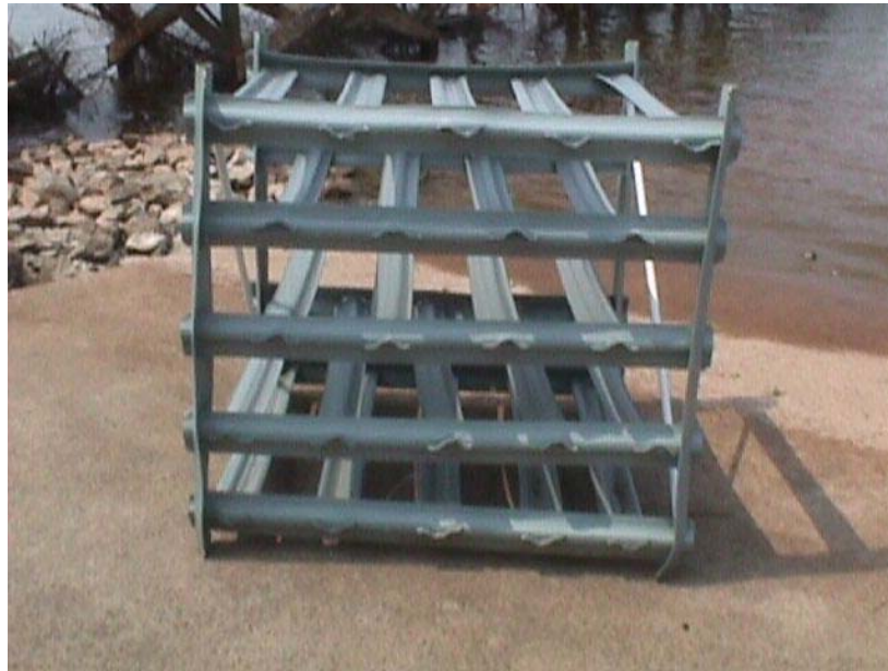
Figure 2a: Hab module used as a pier modification structure in an effort to enhance a subset of piers on Fishing Creek Reservoir and Lake Hickory.
