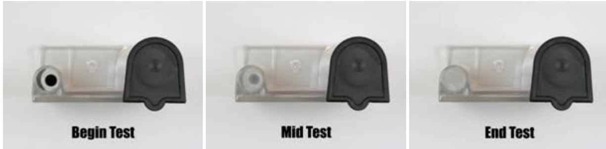
Figure 4. These pictures show the process of the turbidity test for reading cyanuric acid levels in the Taylor K-2005 complete test kit
