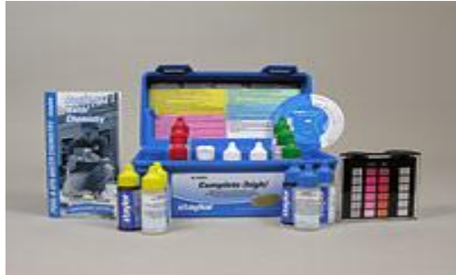
Figure 3. Wake County inspectors test kit for commercial swimming pools. Picture from Taylor Technologies website of K-2005 Complete Test Kit.
