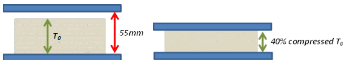
Figure 6.1: the schematic of the compression procedure on Instron
