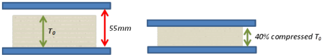
Figure 3.1: schematic of the compression procedure on Instron
