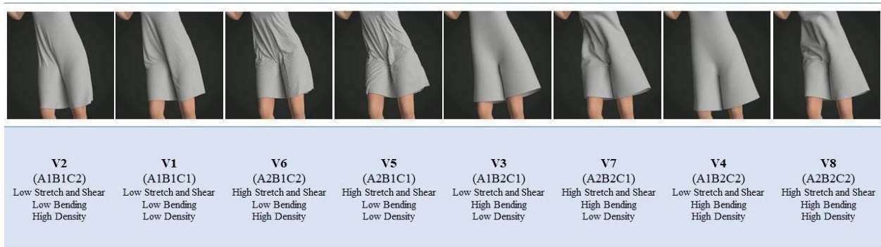
Visual Ranking of Virtual Fabrics Based on Perceived Flexibility (Most to Least)
