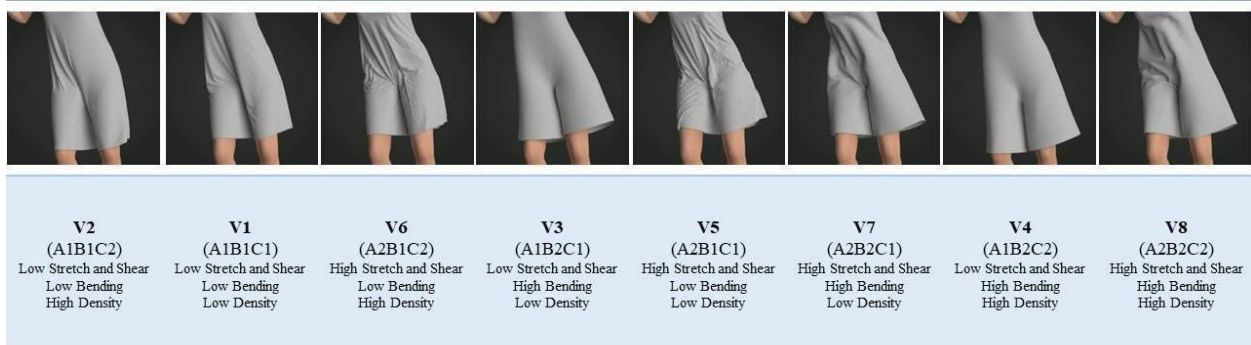
Visual Ranking of Virtual Fabrics Based on Perceived Comfortability (Most to Least)
