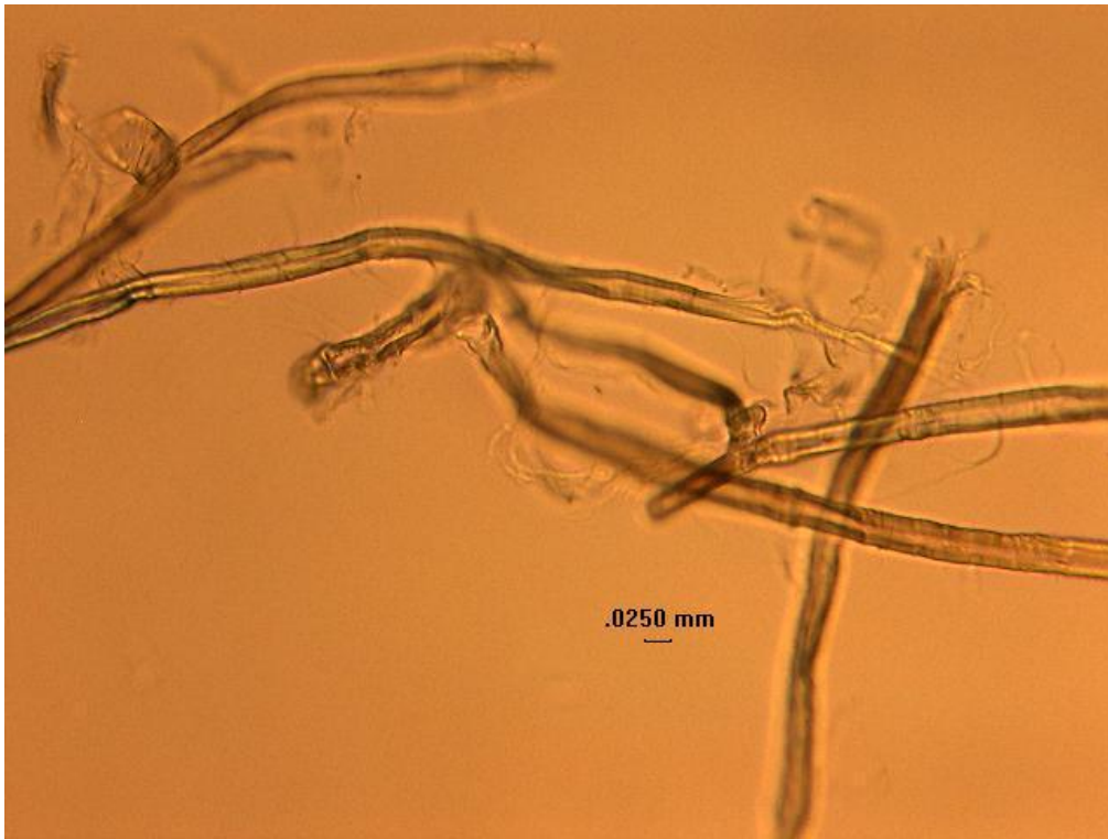
Figure 5 Micrograph of highly refined kraft fibers after 9 hours enzymatic treatment.
