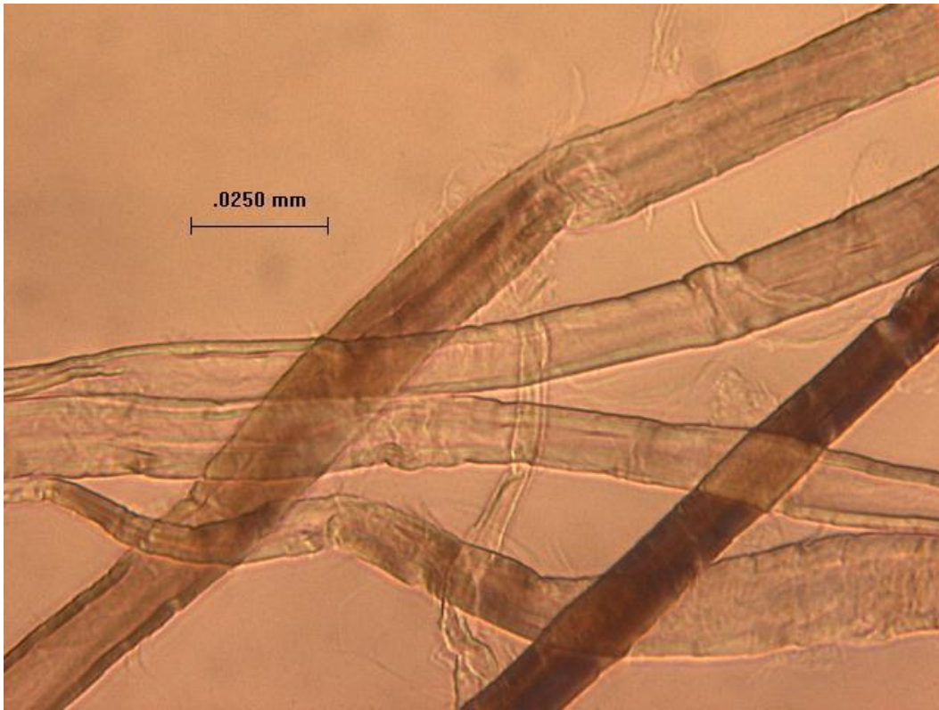
Figure 7 Micrograph of highly refined kraft fibers after 24 hours enzymatic treatment.
