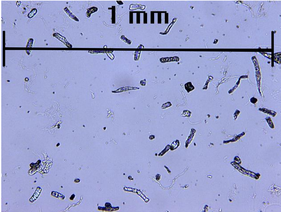
Figure 1 Micrograph of primary fines (collected before refining) from bleached hardwood kraft pulp.
