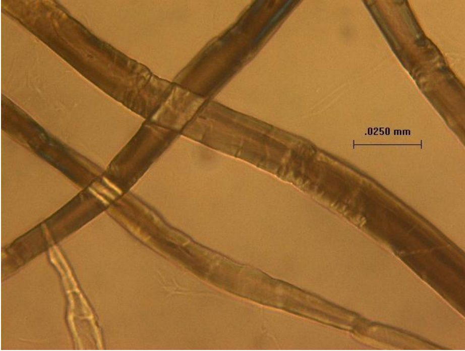
Figure 2 Micrograph of default fiber (collected before refining) from bleached hardwood kraft pulp.
