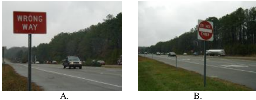
Figure 12: Rear Facing 'Wrong Way' and 'Do Not Enter' Signs
