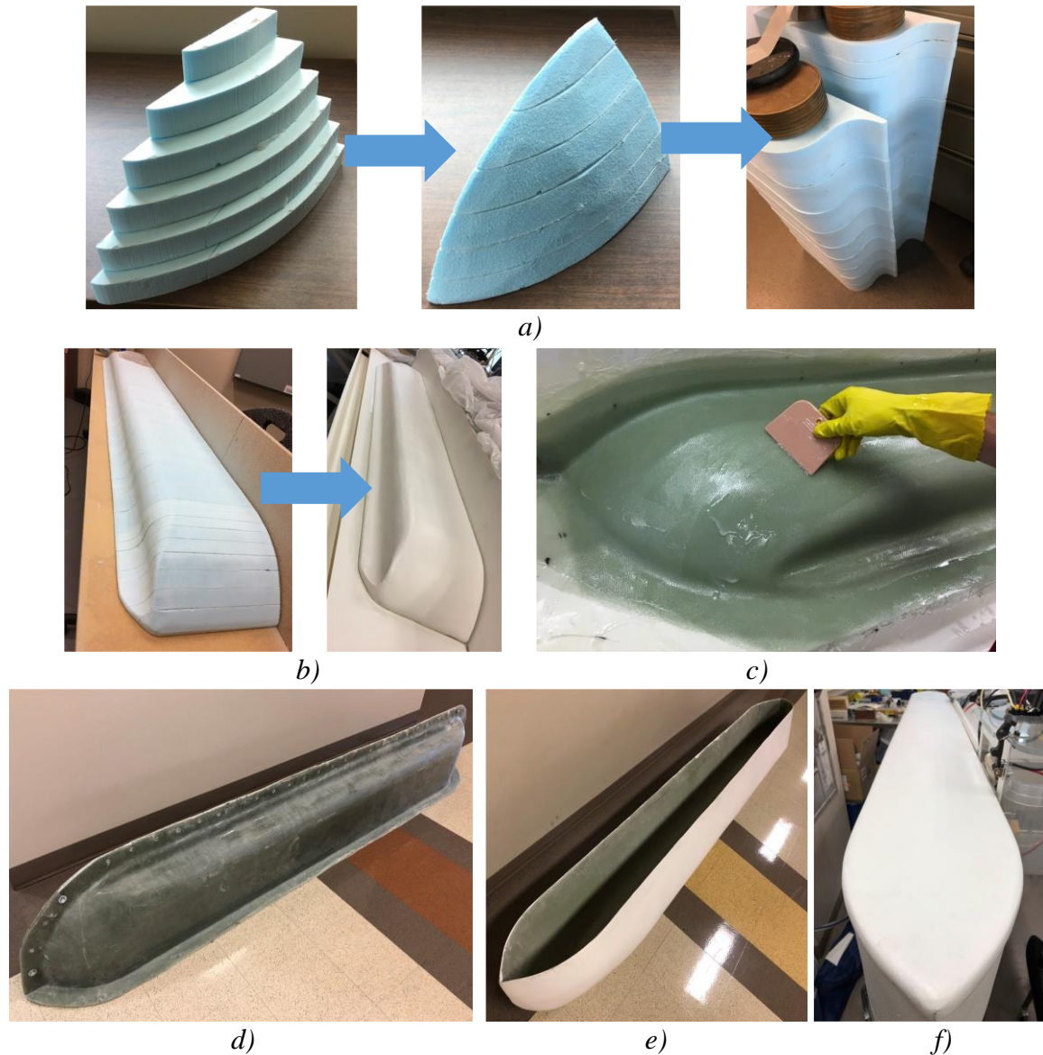
Figure 6. Fabrication of fiberglass pontoons: a) cutting, sanding, and bonding polystyrene plug sections; b) epoxy coating, sanding, and gel-coating of plug; c) fiberglass lay-up of mold over polystyrene plug; d) assembly of mold halves (shown with keel upward); e) fiberglass pontoon after lay-up inside mold an application of multiple finish coats; and f) separately cast pontoon cap installed.
