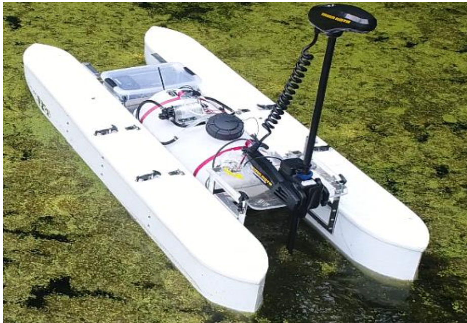
Figure 5. Autonomous boat prototype for identification and chemical treatment of invasive aquatic plant species.
