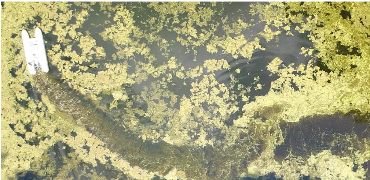
Figure 18. Treatment of watermeal infestation in a small pond using manual navigation and minimal prop submersion.
