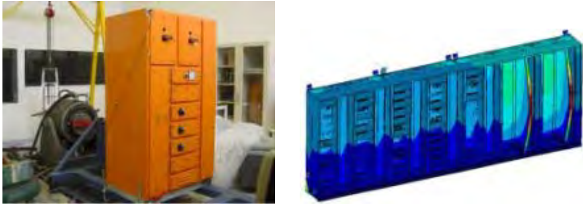
Figure 16 – Switchboard Seismic Test and Switchboard FEA model
