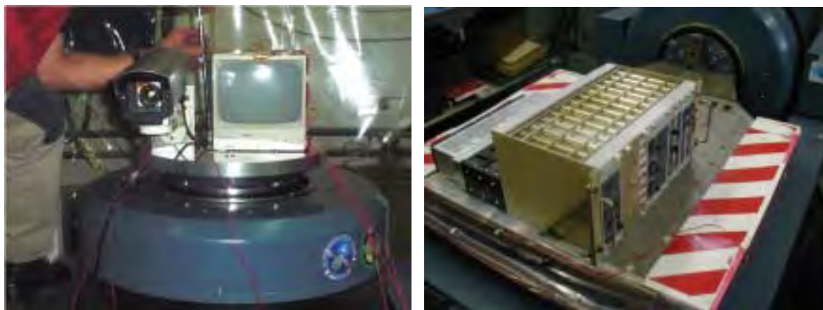
Figure 15 – I&C equipment tests – TV monitor, camera and electronic components in racks
