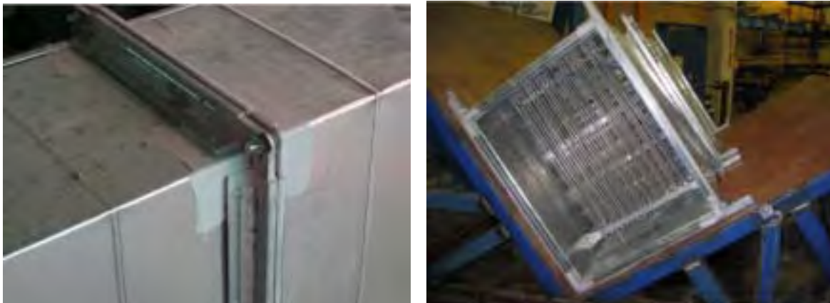
Figure 19 – Ducts mounting and Heater & Damper test
