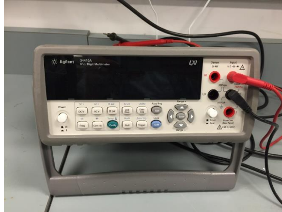
Figure 30. Agilent 34410A 6 \frac{1}{2} digital multimeter.
