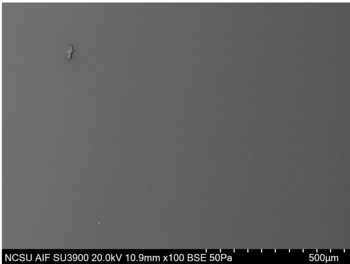
Figure 5.4 SEM image of SbQ-PVA coated on glass
