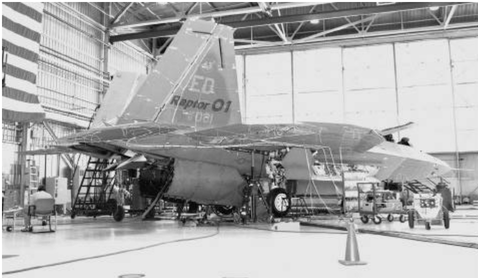
Figure 1.5 Ground Vibration Test of F-22 Aircraft at Edwards Air Force Base (US Air Force Photo)
