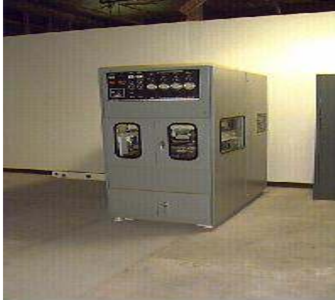
Figure 2-1 Asphalt Pavement Analyzer (APA)
