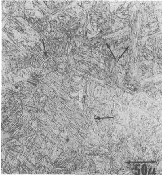
Fig. 7. Optical micrograph of an Fe-Ni cryogenic steel showing grouping of laths into packets.
