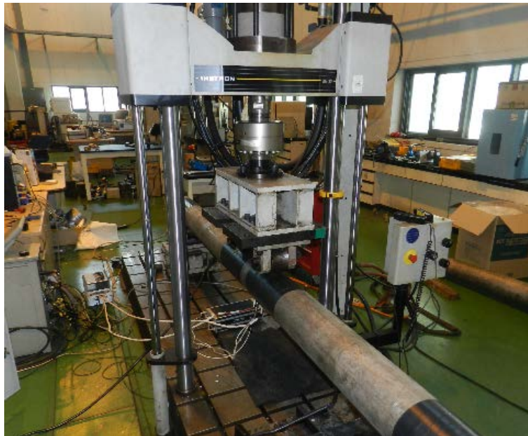
Figure 4. Four-point bending testing system
