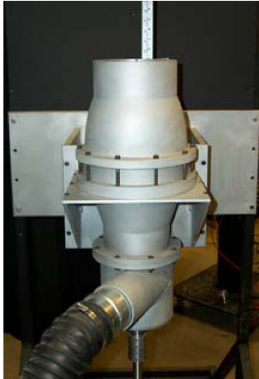
Figure 4-2: Co-flow burner configured for basic experiments
