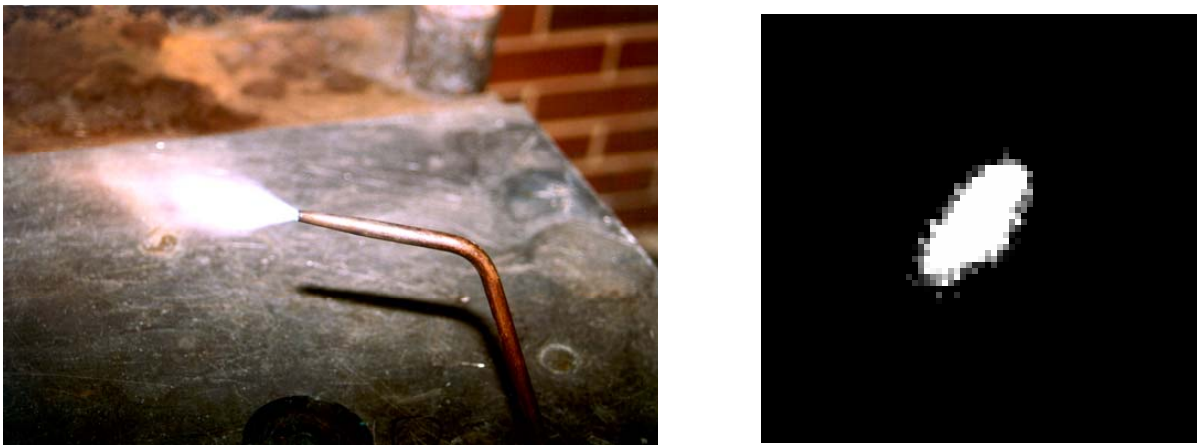
Figure 15: A visible image of an oxy-acetylene torch (left), as well as an image of its UV emission (right).
