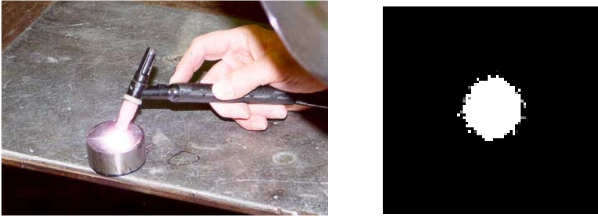
Figure 14: A visible image of a tungsten-inert-gas (TIG) arc welder (left), as well as an image of its UV emission in the range of 320-365 nm (right).
