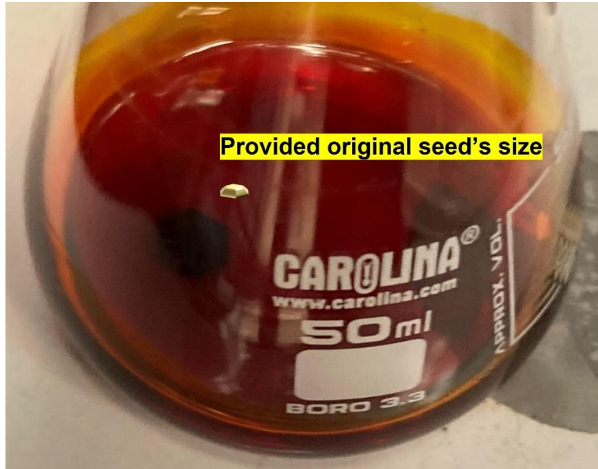
Figure A.2 Growth result of \text{FA}_3\text{Bi}_2\text{I}_9 perovskite single crystals using solution evaporation method with seed, whose size is approximately illustrated.
