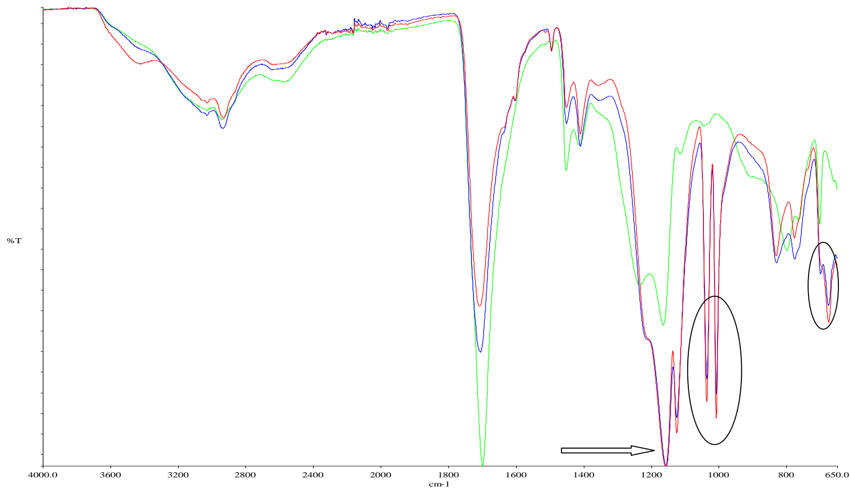
Figure 4.6 FTIR spectra of copolymer including 10 mole% styrene and 0, 15 and 20 mole % styrene sulfonic acid (Green: 10AA90S10I45, Blue: 10AA75S10SSA15I23, Red: 10AA70S10SSA20I23)
