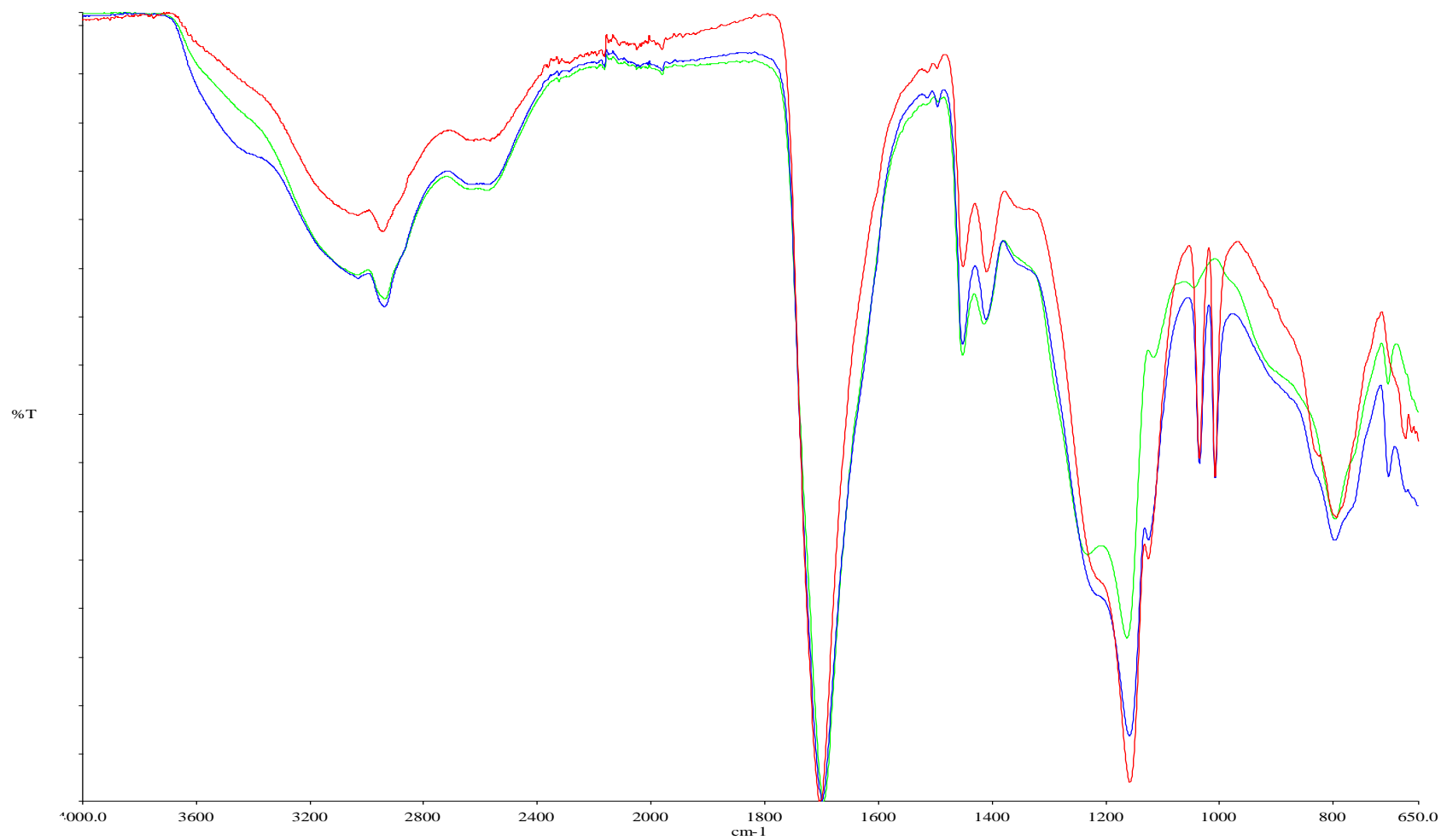
Figure 4.5 Comparison of FTIR spectra of copolymers that has 5 mole % styrene and 0, 5 and 7 mole % styrene sulfonic acid (Green: 10AA95S5I45, Blue: 10AA90S5SSA5I23-3 rd , Red: 10AA88S5SSA7I23)
