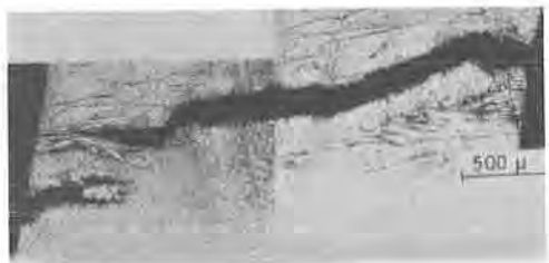
Fig.6 Microstructure of TIG weld metal after creep testing with internal pressure of 3.36 MPa, at 900°C and for 85 hours.
