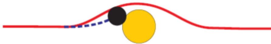
Figure 2-2 Inertial impaction in air filter media(NIOSH, 2003)
