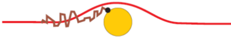
Figure 2-3 Brownian diffusion in air filter media(NIOSH, 2003)
