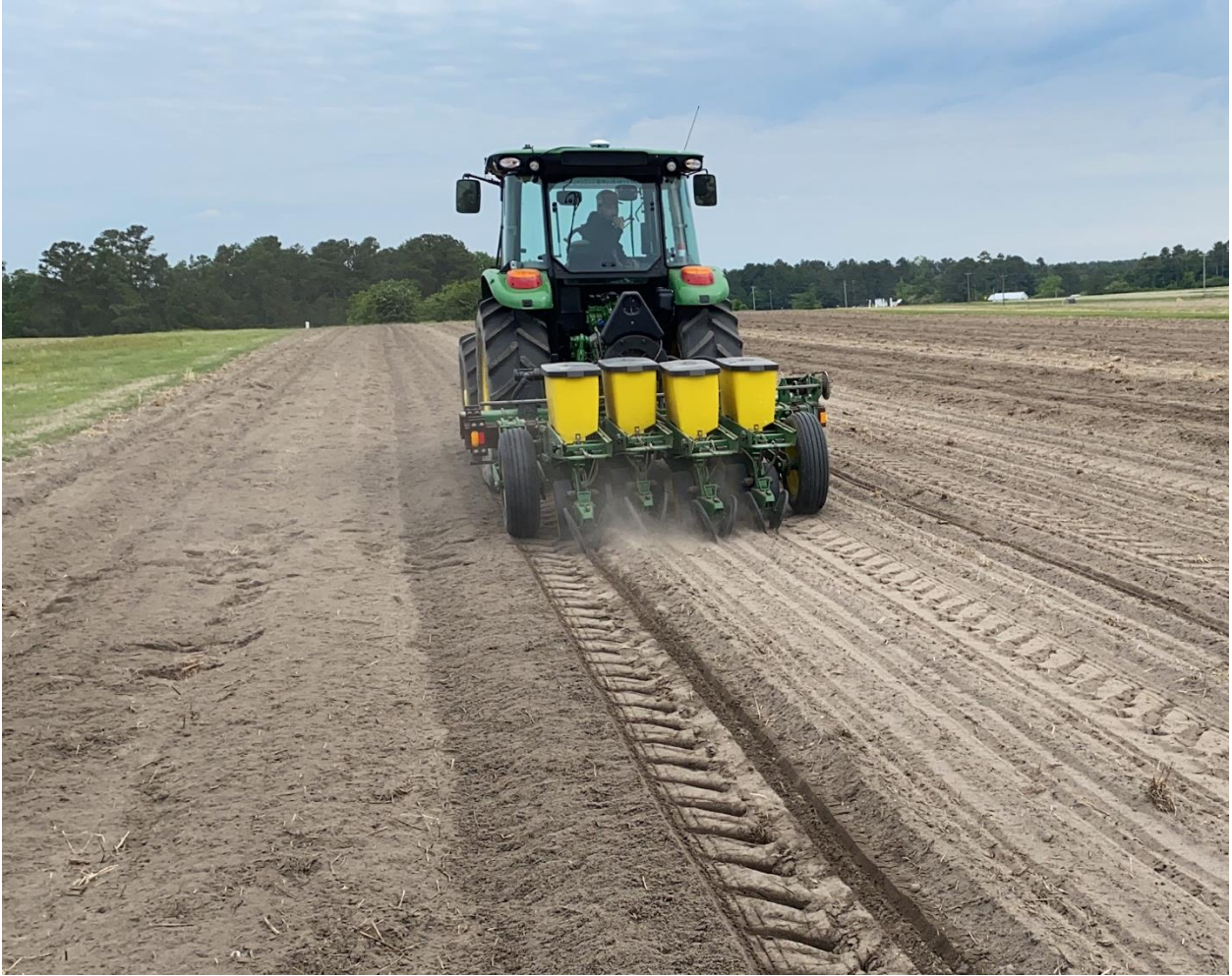
Figure 1. Narrow row John Deere 7200 vacuum planter technology.
