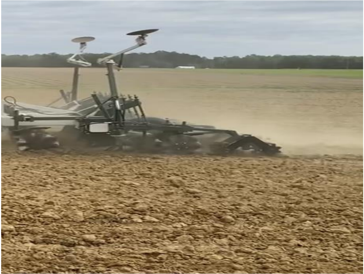
Figure 3. Ripper technology used in front of wide row spacing treatment.
