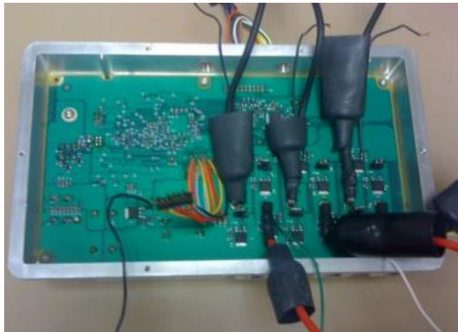
Figure 15 (b): SRM Inverter and controller module. [4]
